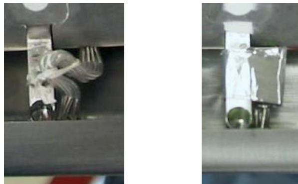
Figure 5: Attachment of slat pressure tube bundles (left) and test quads (right) to a slat track in the experimental model. [3]
