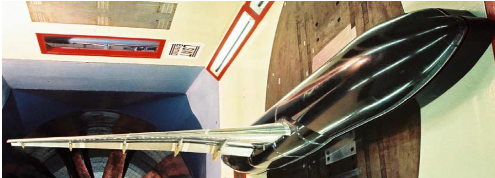
Figure 3: Experimental model of the DLR-F11 wing-body high lift configuration. [3]
